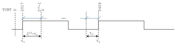
The program also records the number of Timer overflows (rolling from \$FFFF to \$0000). In this particular case, the Timer overflows 3 times between  $t_1$  and  $t_2$ .
